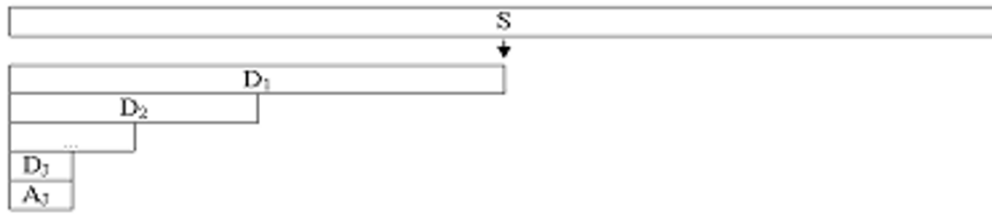
Figure 1 Wavelets transform of a sequence S, with D as details, A as an approximation, and J as level of wavelets analysis.
